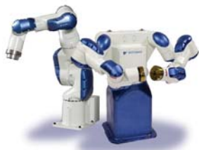
15. A quantum leap in robot technology: single- and dual armed robot models with all the supply cables hidden in the robot arm itself.
