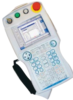
17. All operator controls are located on the programming pendant, often reducing the need for separate PLC and HMI.
