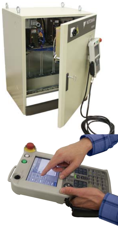
14. The NX100 programming pendant has a touch screen display and is based on Windows CE operative system.
