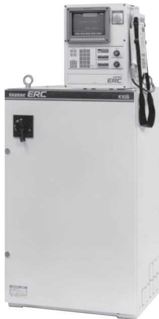
9. The ERC control cabinet with the operator's panel on top.
