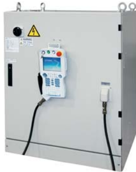
16. The energy saving DX100 controller features faster processing speeds, advanced robot arm control and a robust PC architecture with built-in Ethernet.
